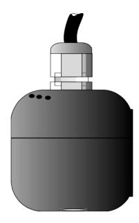
The OxyGuard Probe is a membrane covered galvanic cell that generates an electrical signal proportional to the oxygen pressure it senses, no matter whether it is in water, air, gas, wine, oil or something else. The probe can be used to measure dissolved oxygen in aquaculture, the environment, in clean water, waste water and in oil or other fluid. It can measure very small oxygen concentrations in inert or explosive gases as well as the oxygen content of ambient air and the purity of oxygen gas.
