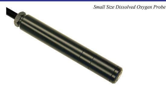
The OxyGuard Mini Probe is a membrane covered galvanic cell that generates an electrical signal proportional to the oxygen pressure it senses, whether it is placed in water, air, oil, wine etc..
