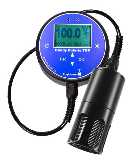
The OxyGuard Handy Polaris TGP (Total Gas Pressure) is a hand-held gas pressure meter. It can operate in three modes, one where it acts as a standard Handy Polaris dissolved oxygen (DO) meter, one where it is a total gas pressure meter that shows pressures as percent saturation values and one where it is a total gas pressure meter that shows pressures as volume percentages.
