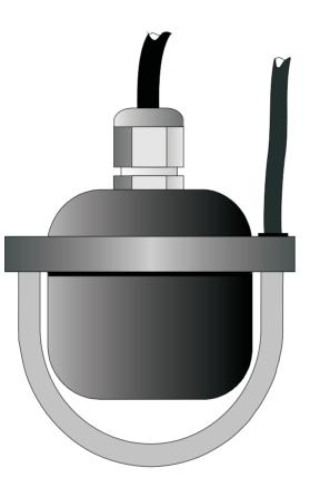
The **OxyGuard OxyClean** is a small attachment with a large effect for use with OxyGuard dissolved oxygen probes! Compressed air is used, and a blast of air of a few seconds is enough to clean deposits from the membrane amazingly efficiently. This short blast of air is hardly enough to disturb the measurement, and blowers controlled by the oxygen measurement will not normally be affected.
