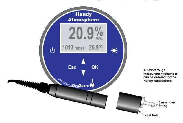
The Handy Atmosphere is a hand-held meter designed to measure oxygen in gas. It can be used to measure the low oxygen content of packaging gas, the oxygen content of the air and the purity of oxygen gas from oxygen generators and the like. A separate brochure is found for a version designed to measure the oxygen content of the modified atmosphere inside food packages.
